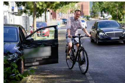
Figure 1: Painted bike lane overlapping with the door zone of parked cars.
